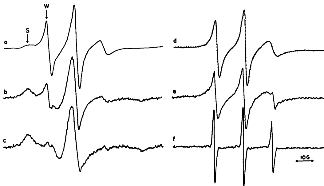
Figure 2. ESR spectra of 5-doxyl stearate in AB:DOC (a-c) and DOC (e-f) systems: (a) 5.0; (b) 1.6; (c) 1.2 mM AB; (d) 6.0; (e) 2.0; (f) 1.0 mM DOC. S and W indicate the low-field components of the spectra due to strongly and weakly immobilized label populations, respectively. The dotted line in d corresponds to the spectrum obtained by subtracting 2c from 2a. NaCl-37 mM phosphate buffer, 300 mOsm, pH 7.4. From ref. 29.
